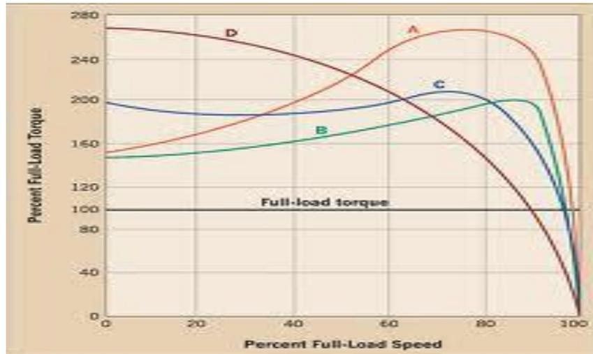
Class B machines should have a lower starting current compared to A (500% rated versus 800% for B)
