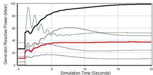
Figure 4: Example 37-Bus Generator Mvar Outputs
