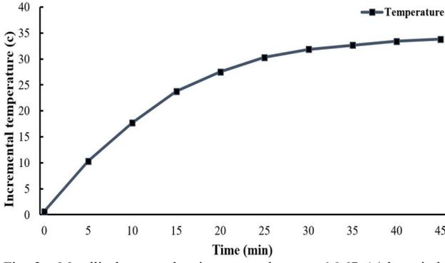
Fig. 2. Metallic hot spot heating curve due to a 16.67 A/phase induced current.
