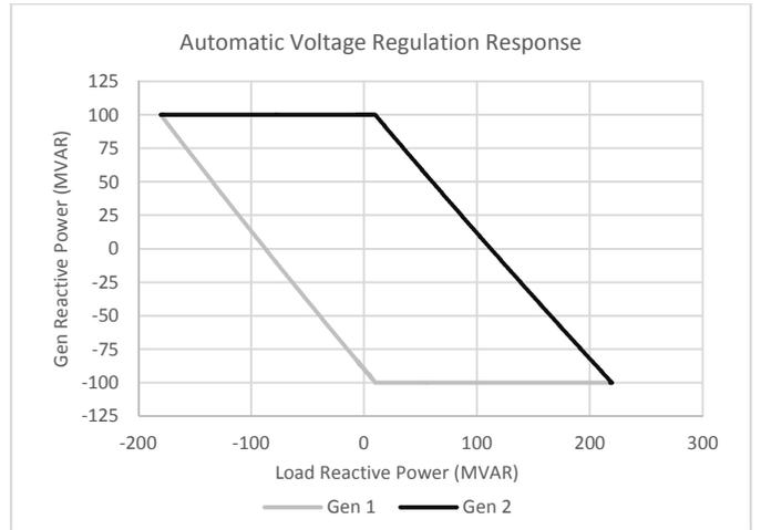
Fig. 9 AVR voltage control response of units 1 and 2
