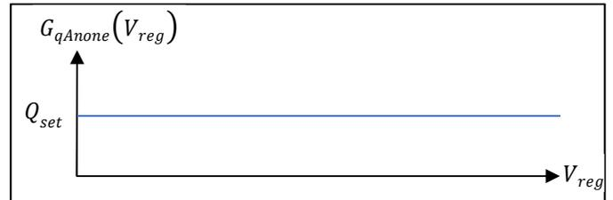
Fig. 6.  $Q(V_{reg})$  for units without voltage regulation
