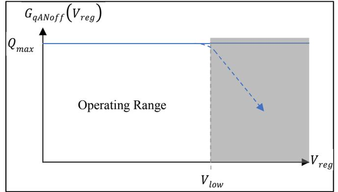
Fig. 5.  $Q(V_{reg})$  for units operating at reactive power limits
