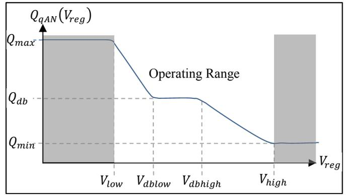
Fig. 4.  $Q(V_{reg})$  for units on Voltage Droop Control
