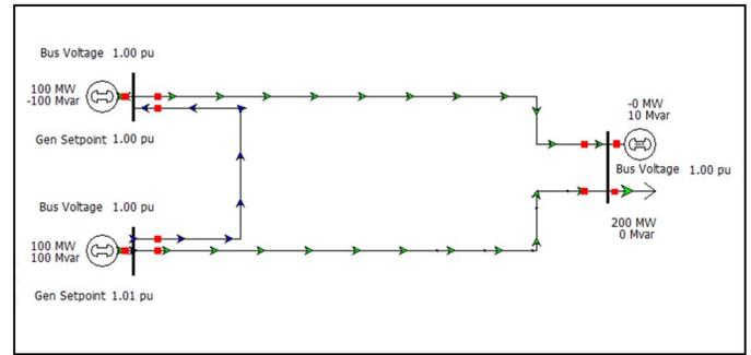
Fig. 10. One Line of case study with generator interference
