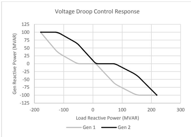
Fig. 8. Voltage Droop Control response of units 1 and 2
