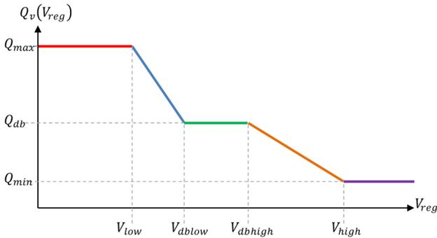
Fig. 2. Voltage Droop Control Q(V) function as defined by user
