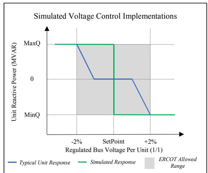
Fig. 1. A simulated Q(V) function and a typical industry Q(V) function
