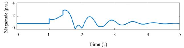
Fig. 6. Generator Internal Current
