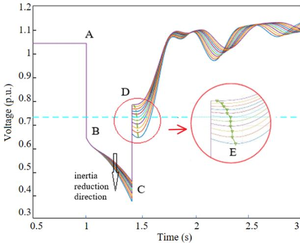
Fig. 1. Bus voltage profiles as inertia varies
