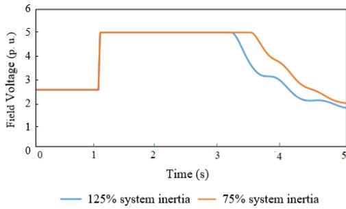
Fig. 4.  $E_{fd}$  values under different inertia values
