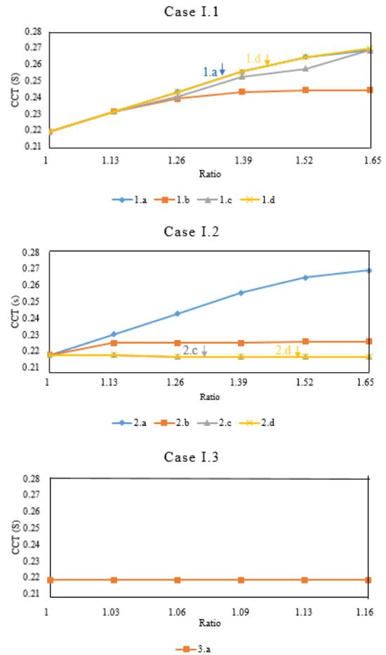
Fig. 8. Multiple CCTs under different inertia scenarios in case set I
