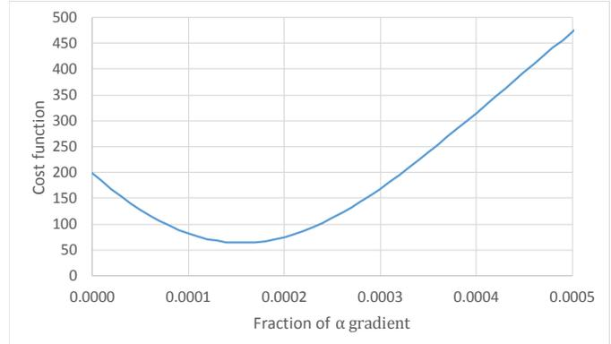
Fig. 1. First VPM iteration of case 5, showing the cost function with respect to the distance in the negative gradient direction.
